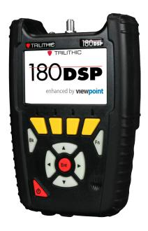
Provides cable installers and field technicians a full complement of RF measurement functions
