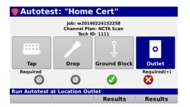
Multi-user support allows technicians that work in various territories to easily switch channel plans, standardized autotest apps, and test limits or login as a completely different user. Connecting to ViewPoint allows techs to upload job data in near real-time as well as transmit and receive channel plans, autotests, and firmware.
